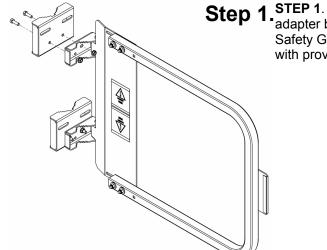
**1. STEP 1**. Attach Large Pipe adapter bracket to the Ladder Safety Gate mounting bracket with provided bolts.
